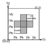
PV-diagram from  $P_1 : P_a P_b V_b V_a$  $P_2 : P_b P_a V_a V_b$  Executions are directed paths – since time flow is irreversible – avoiding a forbidden region (shaded).
