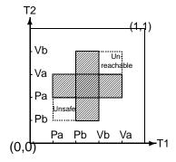
PV-diagram from  $P_1 : P_a P_b V_b V_a$  $P_2 : P_b P_a V_a V_b$  Executions are directed paths – since time flow is irreversible – avoiding a forbidden region (shaded).
