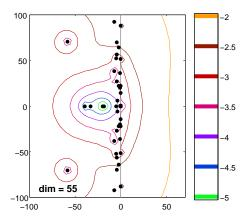
Stable Boing wing flutter matrix. Close-up near eigenvalue with Re  $z\sim 0$
