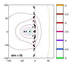
Unstable Boing wing flutter matrix. Close-up near eigenvalue with  $\text{Re}\,z>0$
