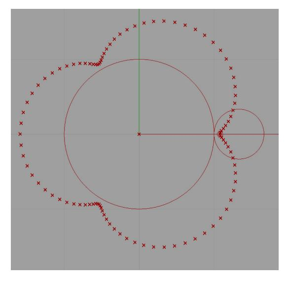
We will produce a visual picture of the epitrochoid curve by drawing a large number *N* of points on canvas tracing out this curve. The epitrochoid curve is generated by a point attached to a circle of radius *r*2 (the rolling circle) rolling around the outside of a fixed circle of radius *r*1, where the point is at a distance *d* from the center of the rolling circle.
